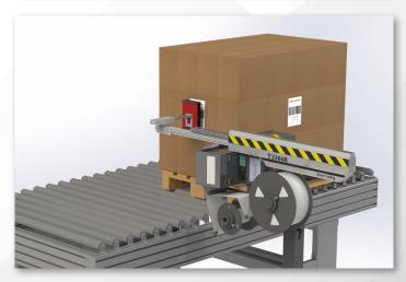
It can be applied on 1, 2 or 3 sides (front - side - rear) with the application equipment located outside the production line and with the product stationary.
